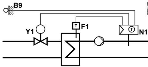
Heat exchanger control through control of the 2-port valve in the primary flow, outside temperature compensation
