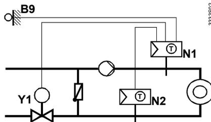
Flow temperature control with maximum limitation of the secondary return temperature in a district heat plant, outside temperature compensation
