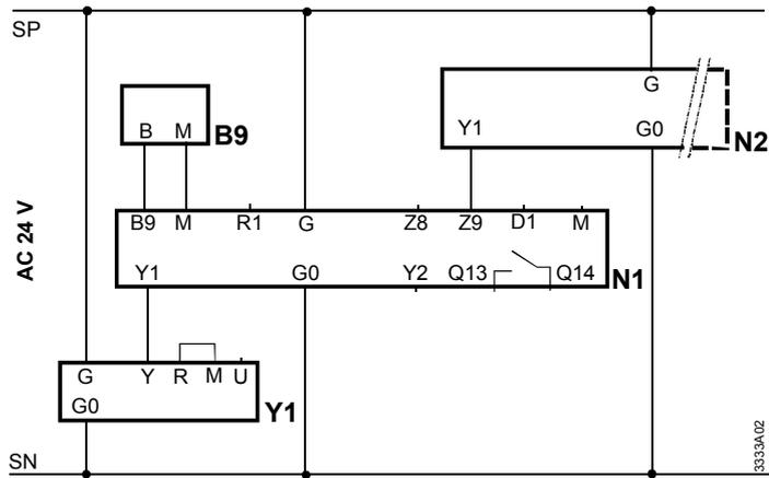
Flow temperature control, outside temperature compensation and maximum limitation of the flow temperature
